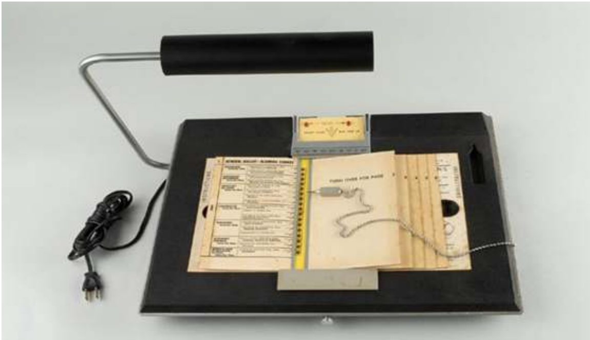
Votomatic Machine: a punch card voting machine originally developed in the 1960s. Courtesy: Wikimedia Commons
